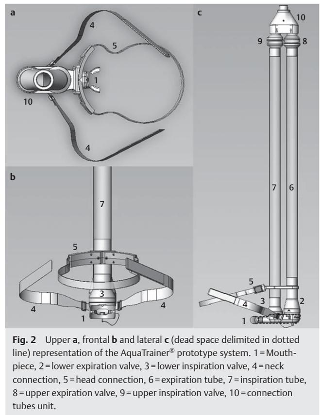
**Fig. 2** Upper **a**, frontal **b** and lateral **c** (dead space delimited in dotted line) representation of the AquaTrainer<sup>®</sup> prototype system. 1 = Mouth-piece, 2 = lower expiration valve, 3 = lower inspiration valve, 4 = neck connection, 5 = head connection, 6 = expiration tube, 7 = inspiration tube, 8 = upper expiration valve, 9 = upper inspiration valve, 10 = connection tubes unit.
